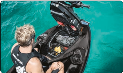
Direct-Access Front Storage All your gear within arm's reach thanks to a 96 L front storage area, easily accessible from a seated position. Simply raise the handlebars to access essentials for any adventure.
